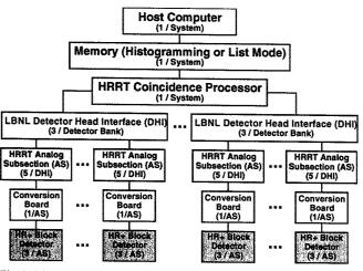
Fig. 3: Diagram of the complete data collection chain, showing the custom LBNL and CTI components and their inter-relations. The camera will use 80 CTI ECAT HR+ block detectors, 28 LBNL conversion boards, 28 CTI HRRT Analog Subsection boards, 6 LBNL custom Detector Head Interface boards, 1 CTI Coincidence Processor and a PC.
