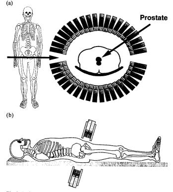
Fig. 2: Positron tomograph for prostate imaging. (a) Drawing of a transaxial view through prostate, showing the patient centered between two detector banks. The individual detector modules are angled to point towards the prostate. (b) Drawing of the sagittal view. The bottom arc is fixed below the patient bed, whereas the top arc adjusts vertically for patient access and compactness. Both detector banks are tilted and positioned as close as
