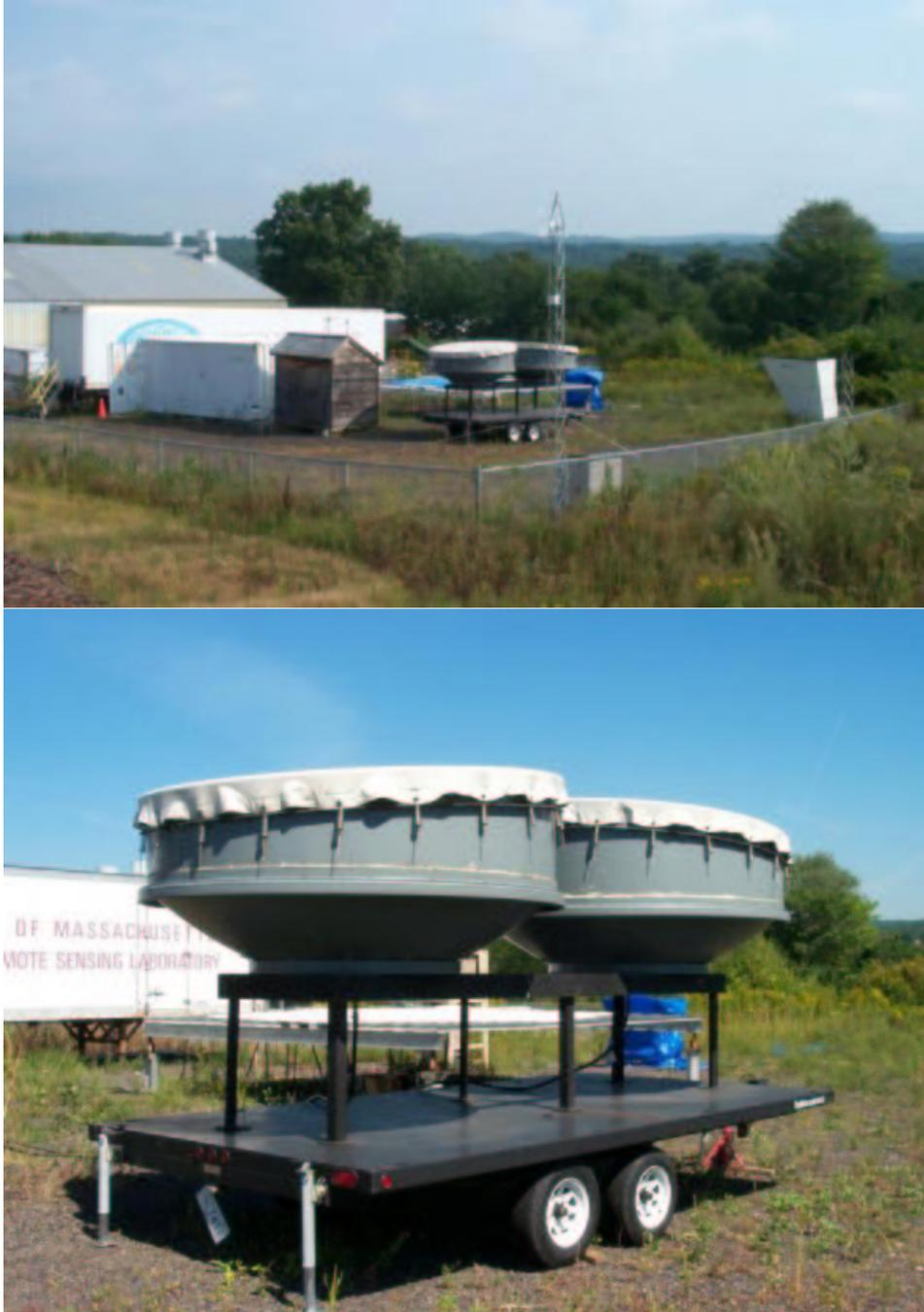
Figure 4: TOP: View of the Tilson Farm field site at UMass. Visible are a 20' tower with a 3D sonic anemometer, a Doppler sodar (on right), FMCW radar, and TEP array (behind FMCW). BOTTOM: Closeup of the FMCW radar antennas.
