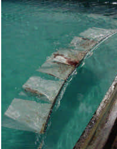
Figure 27. Boom 1: MYCELX Infused PP Felt Boom.
