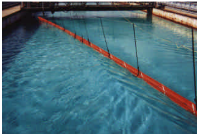
Figure 22. View of Boom, Showing Suspenders.
