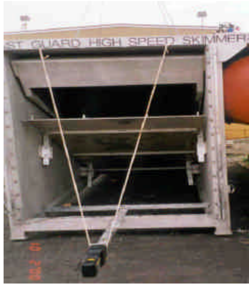
Figure 34. Thickness Gauge Mounted on HSS.
