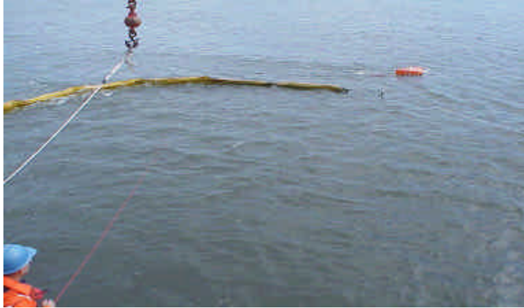
Figure 6. Boom Vane Deployed from Larger Vessel in New York Harbor.
