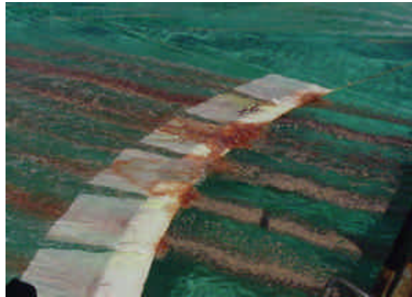
Figure 28. Boom 2: Composite Boom, Tested with Diesel Fuel.
