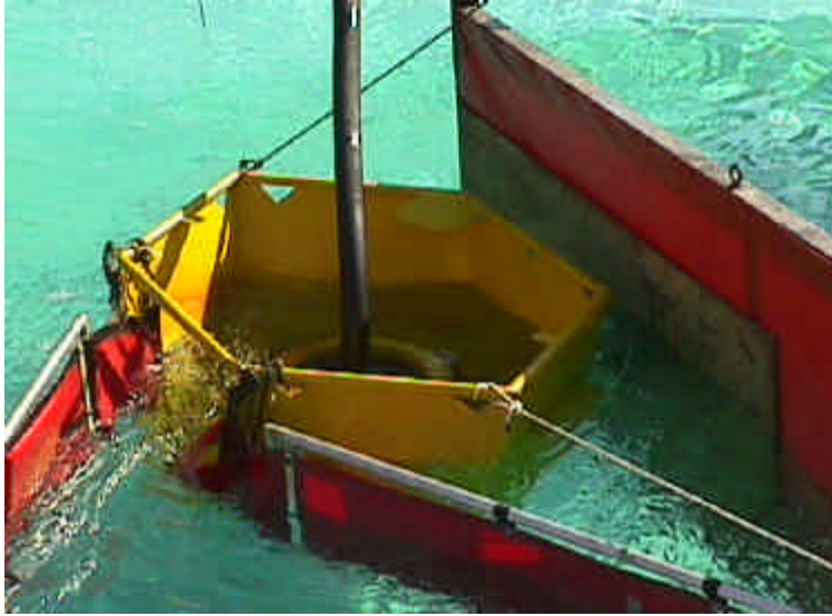
Figure 15. High Speed Circus Collector.
