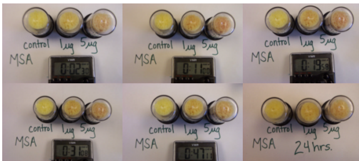
Figure 16. Colorimetric response of Yellow to Red Sensor version (for MSA)
