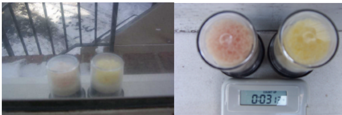
Figure 26. Detection of DFP on frozen surface at -9^{\circ}\text{C} (left picture 2min, right picture 3min)
