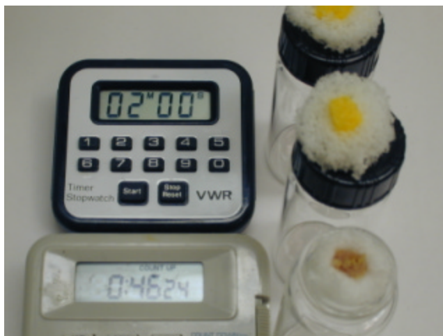
Figure 21. Continuous sensing of DFP in air 45min after activation.
