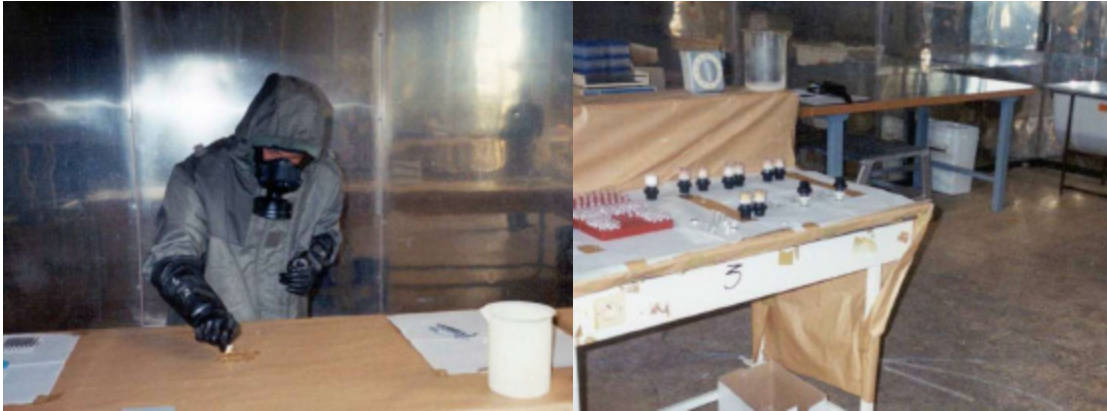
Figure 30. French soldier activating Agentase TLS on table (left) and sensors after testing yielding yellow, green and red colors (right)
