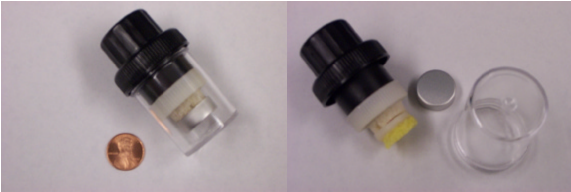
Figure 14. Agentase TLS with aluminum cap attached (left) and removed (right)
