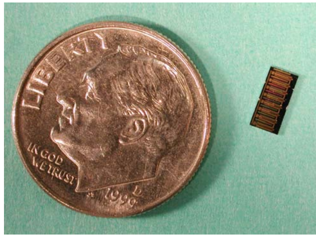
Fig. 5.9: Compact MEMS-based switchable capacitor bank implemented with on-chip MIM capacitors
