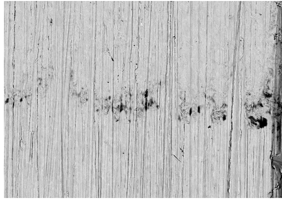
Figure 6. Non-crack damage for 10%-of-life sample at 620 MPa clamping stress. Fatigue loading axis is vertical.
