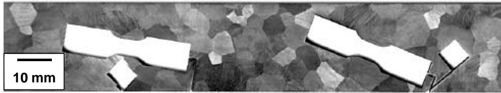
Figure 2: Machining blank. Note the large grain size of material used in specimen manufacturing.
