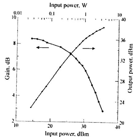
Fig. 3. Output power and gain versus input power.
