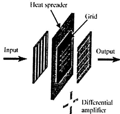
Fig. 1. Schematic of the grid amplifier with heat spreader. The input and output waves are in orthogonal polarizations.
