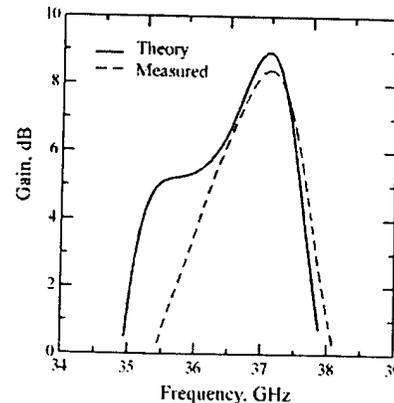
Fig. 4. The theory and measurement of small-signal response of the grid amplifier. They agree with each other except around 35.5GHz.
