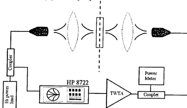
Fig. 7. Focused beam measurement system.
