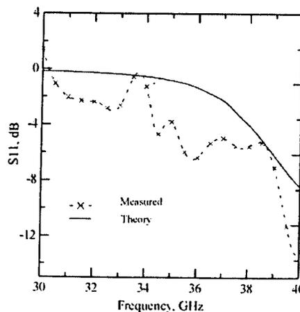
Fig. 8. The measured and theoretical reflection coefficients.
