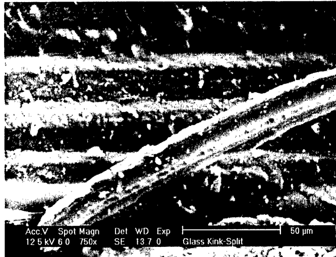
a) A high magnification view of a broken glass fiber
