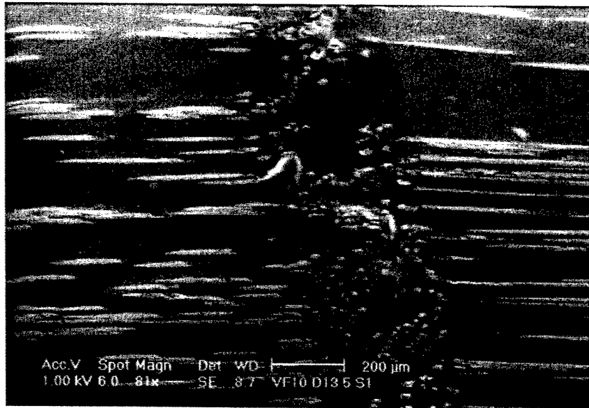
Figure 7.2: Kink band in glass composites of fiber diameter 13.5\mu m and V_f = 10\%
