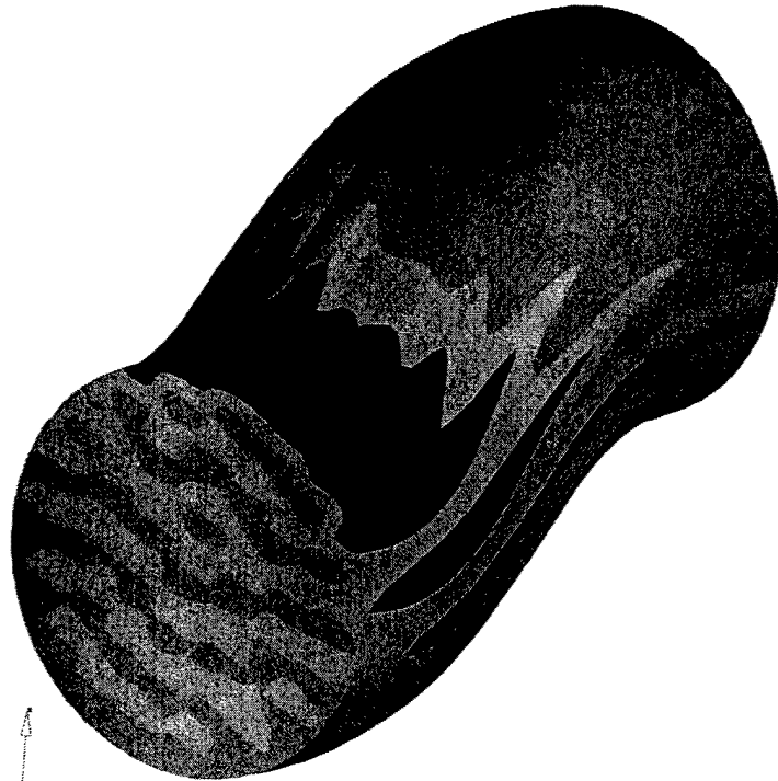
Figure 5.17: Contours of \epsilon_{xx} for the carbon/vinylester composite of V_f = 0.5 and \phi_1 = 1^0 with orthotropic fiber properties
