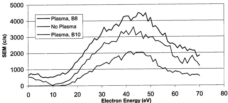
**Figure 9.** Accumulated electron energy scan for  $\text{NO}_2$  ( $m/z=46$ ) for plasma exhaust from APD210 Test Device 8 at 14 kV, 6kHz; APD210 Test Device 10 at 12.8 kV, 5 kHz; and background (no plasma). (Plasma device located ~3" from EQP) (ref. exp. 9 & 10)
