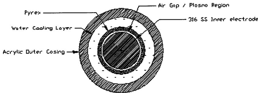
**Figure 4. Cross-sectional drawing of the APD 210.**
