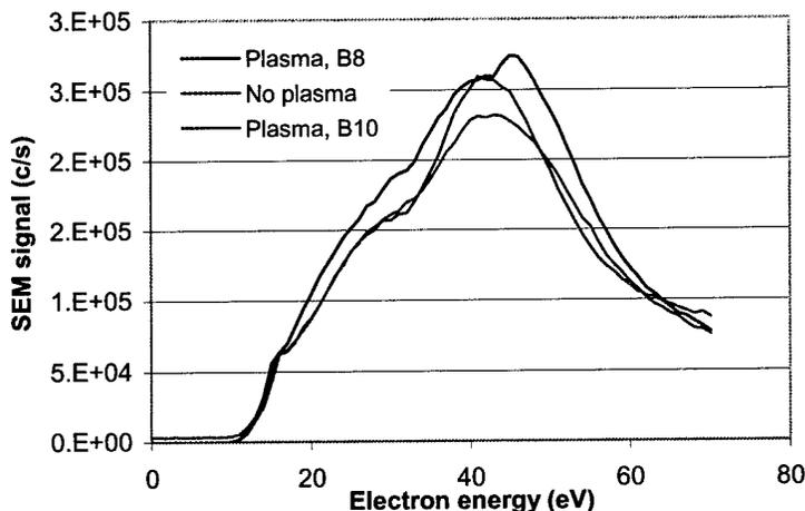
Figure 8. NO ( $m/z=30$ ) accumulated electron energy scans for plasma exhaust from APD210 Test Device 8 at 14 kV, 6kHz; APD210 Test Device 10 at 12.8 kV, 5 kHz; and background (no plasma). (Plasma device located ~3" from EQP). (ref. exp. 9 & 10)
