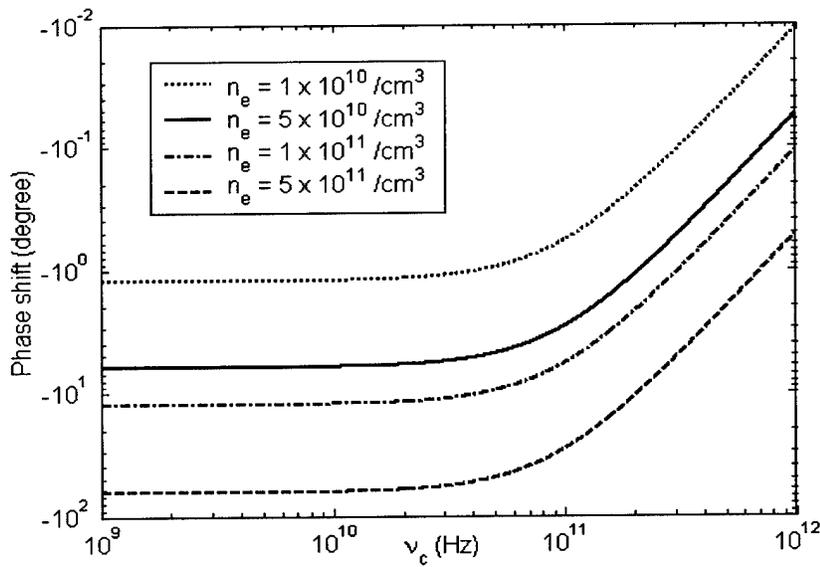
Figure A 8: Phase Shift versus Collision Frequency
