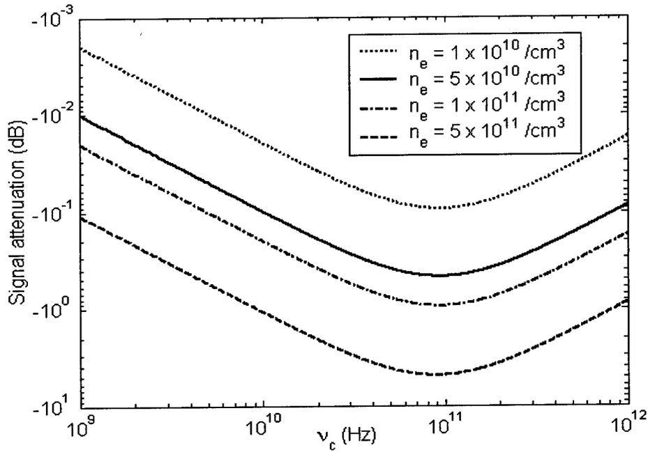
Figure A 7: Attenuation versus Collision Frequency
