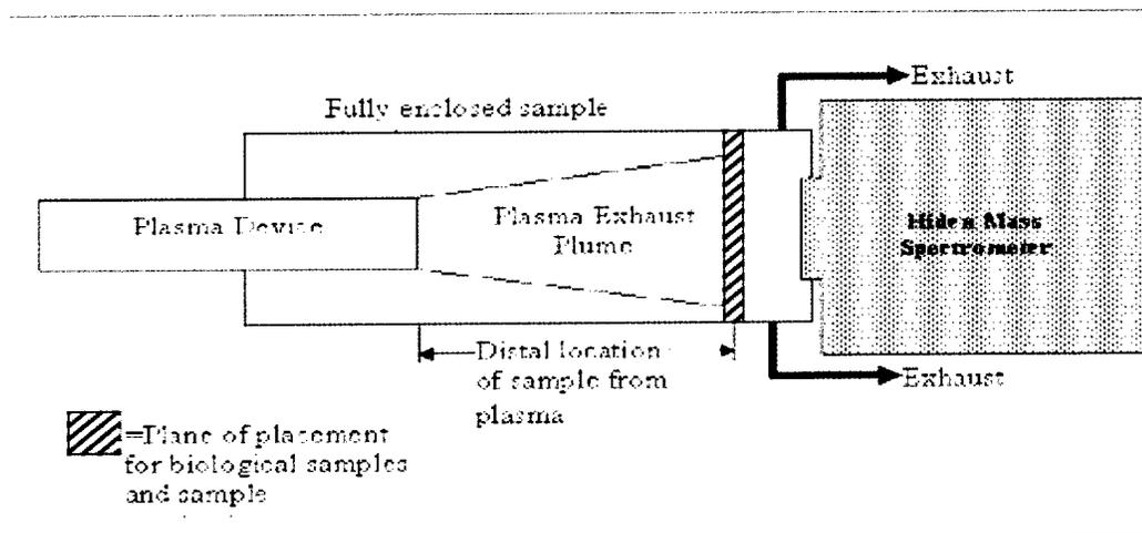
**Figure 7. 2-D Schematic of the Sample Exposure Chamber.**
