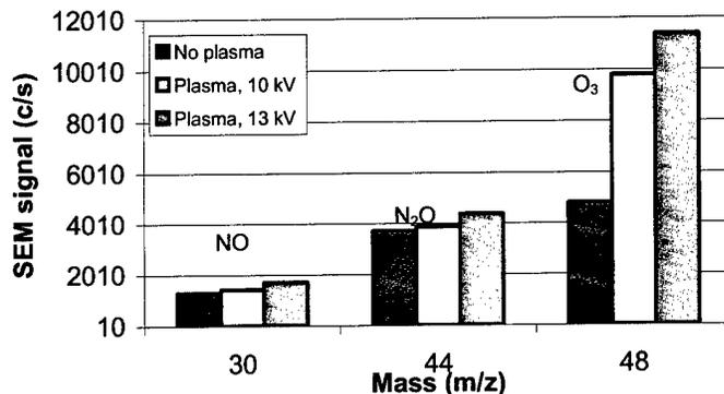
Figure 7. Qualitative signal from the EQP for masses of interest ( $m/z=30, 44, \text{ and } 48[x10^2]$ ) for the baseline case -no plasma- and plasma exhaust from the APD210 Test Device 10 at applied voltages of 10 kV and 13 kV (both at 2 kHz).
