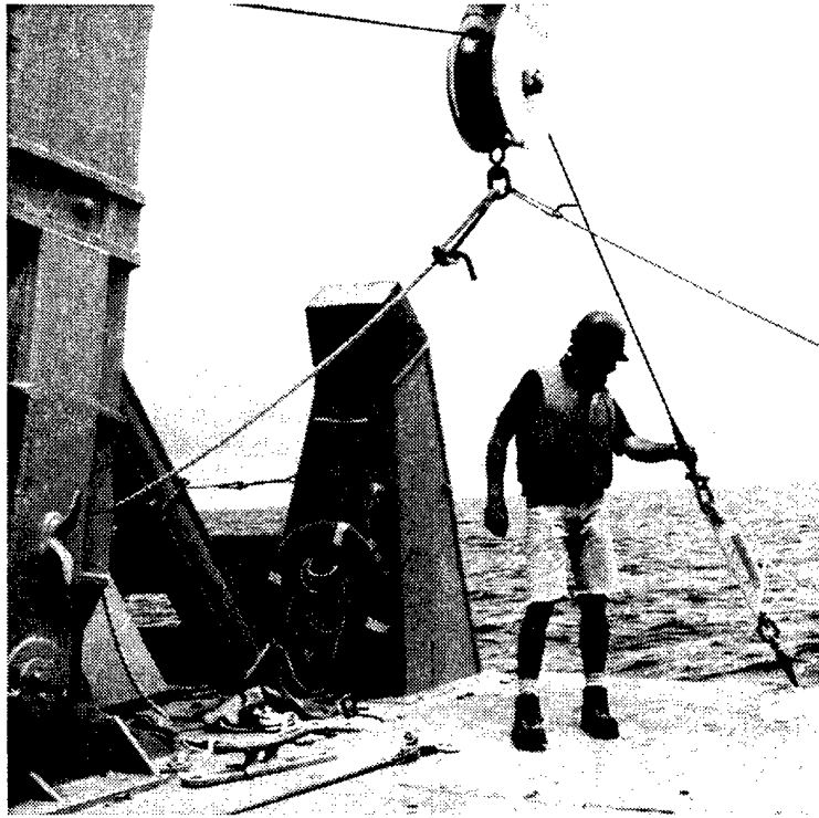
Figure 14: Using the hanging block to control instrument deployment.
