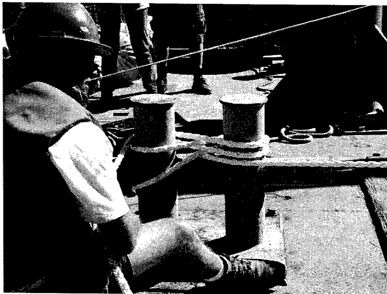
Figure 15: H-Bit rigged for deploying 2000 meters of line.
