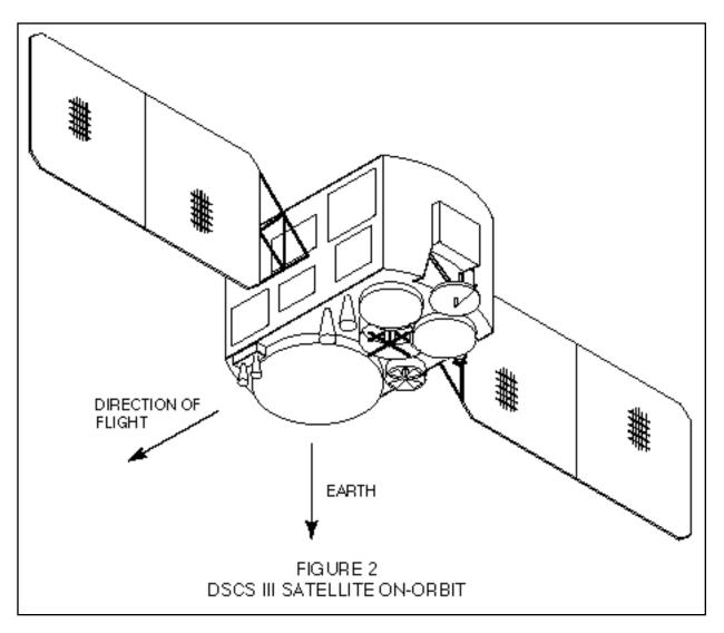
The structure consists primarily of aluminum honeycomb panels joined with magnesium and aluminum edge members. Two equipment panels are manufactured from thoriated magnesium (ionizing radiation source).
