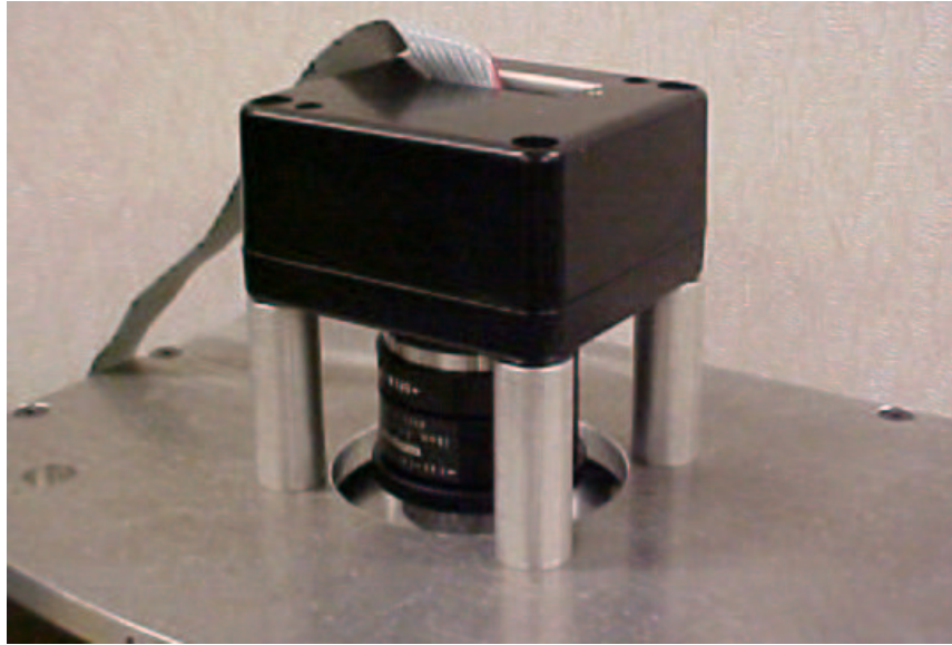
Figure 4.7 Digital Camera in Modified Mounting Position
