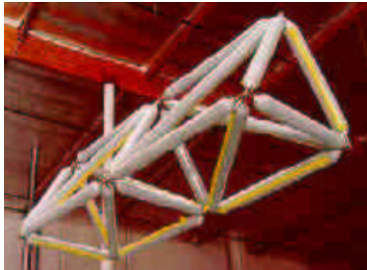
Figure 2.5 L'Garde Inflatable Space Truss
