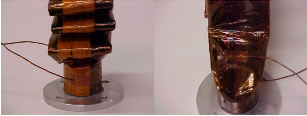
Figure 4.3 Tube Thermocouple Locations
