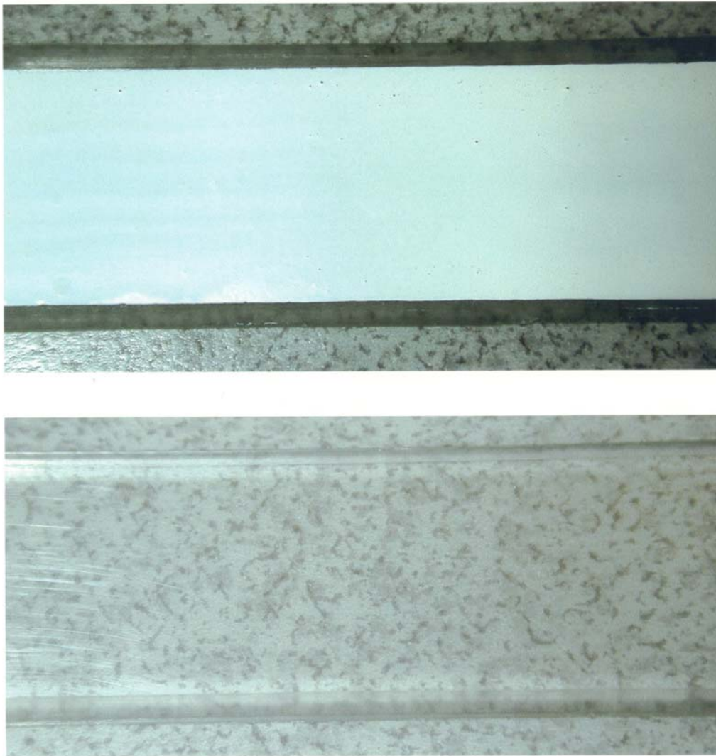
Figure 4: Polycarbonate annular reactor coupons used in the biofilm prevention study; the coupons contain the biocidal polyurethane coating (top) and no coating (bottom).
