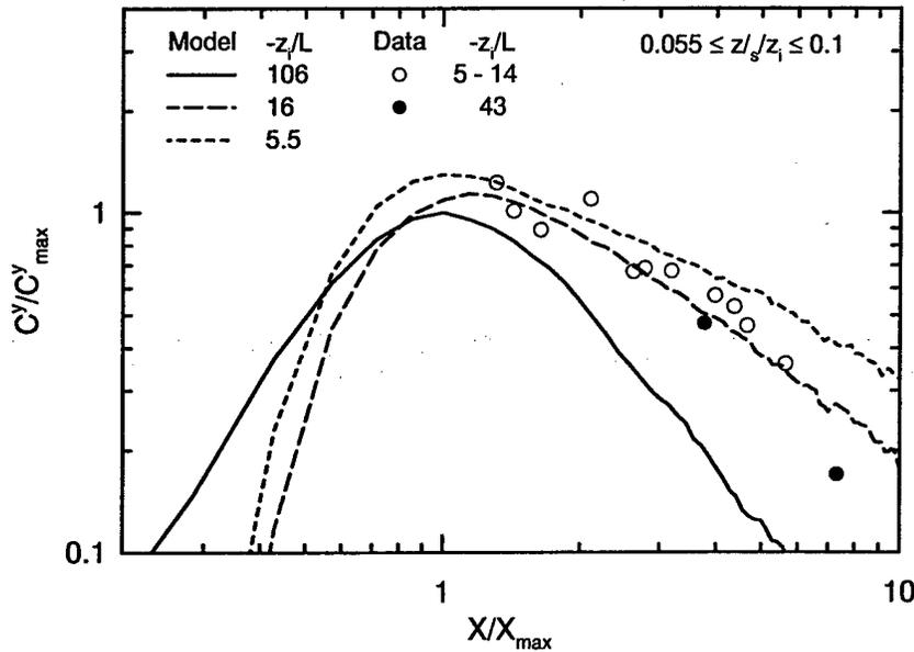
Figure 6: Modeled mean surface CWIC nondimensionlized by the maximum surface CWIC,  $C_{max}^y$ , as a function of  $X/X_{max}$ , where the  $C_{max}^y$  and  $X_{max}$  here correspond to the case  $-z_i/L = 106$ ; the field data (Gryning and Lyck, 1984) are downwind of a 115-m source in the CBL surface layer.
