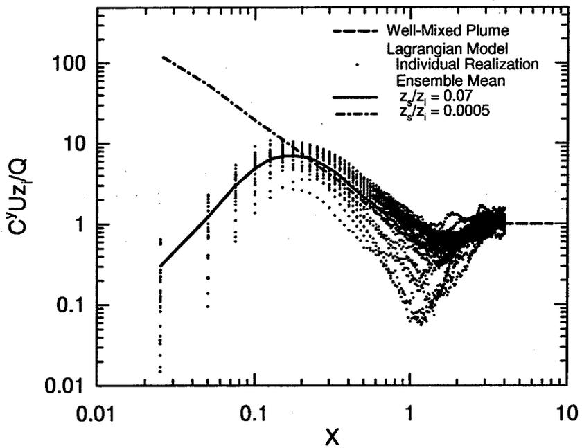
Figure 10: Dimensionless CWIC at the surface versus dimensionless downwind distance for an elevated source ( $z_s/z_i = 0.07$ ) in the surface layer; modeled mean and individual realizations of the CWIC.
