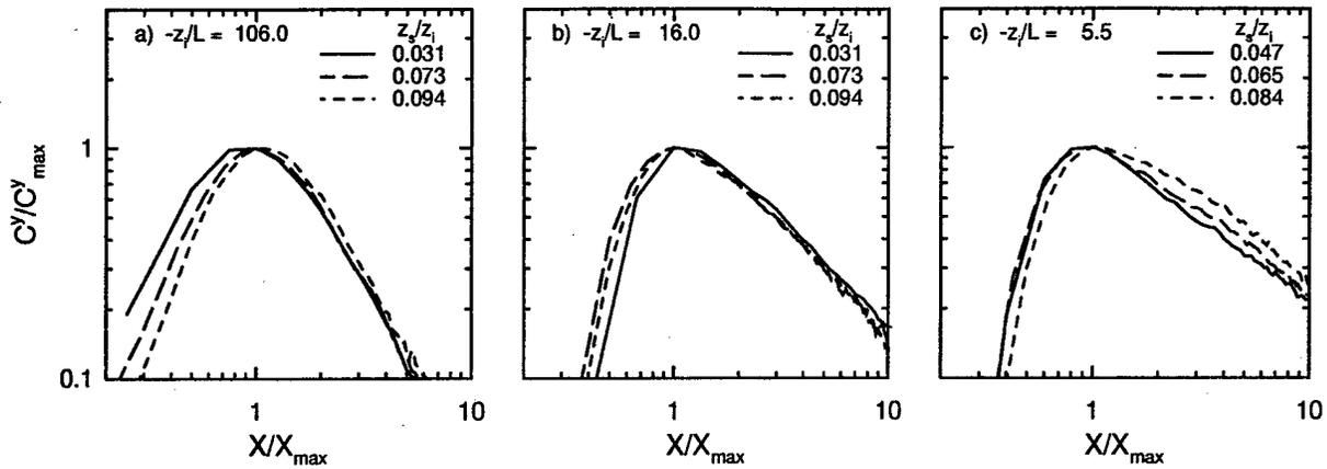
Figure 5: Surface CWIC scaled by its maximum value as a function of dimensionless distance ( $X$ ) scaled by the distance to the maximum for three source heights in the surface layer and three CBL cases.
