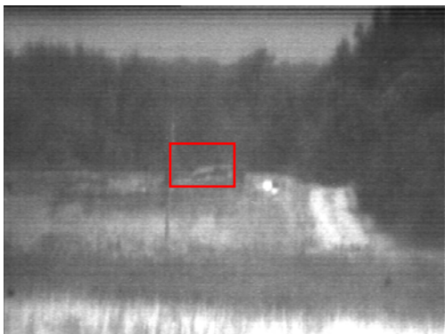
Fig. 1c Image at 660 nm with truck revealed under camouflaged net
