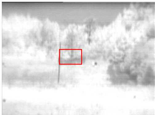
Fig. 1d Image at 780 nm revealing camouflaged net against background
