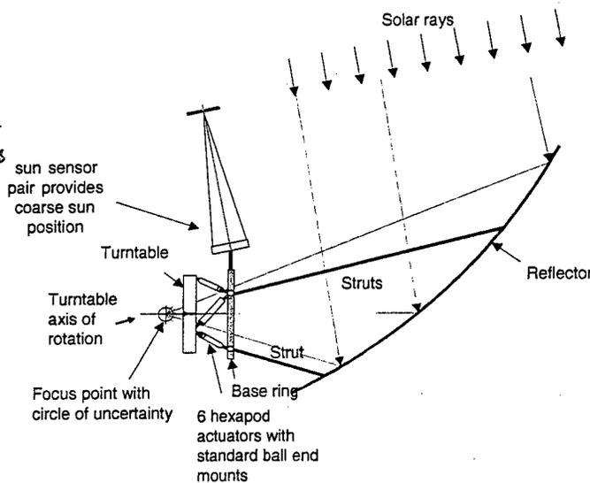
Figure 14. Sun Tracking and Fine Focus Concept
