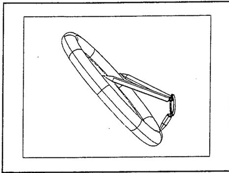
Figure 7. Solid Model of Inflatable Concentrator Support Structure
