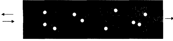
Figure 5. Schematic of coupled quantum dots with discrete impurity sites.
