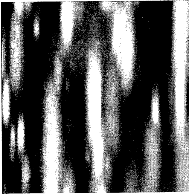
Fig. 9. Atomic force microscope image of older on-axis GaAs surface after homoepitaxial growth. The image is a 3- \mu\text{m} square and the grey scale represents 10 nm with a line roughness of 1.5 nm.
