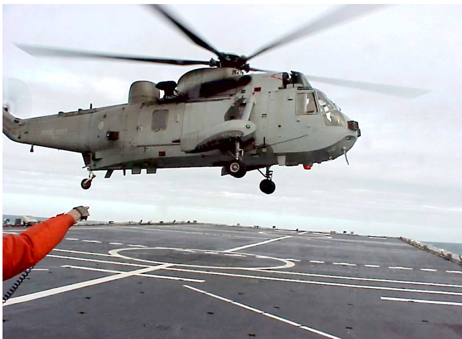
Fig. 10B Cross-deck facing port procedure
