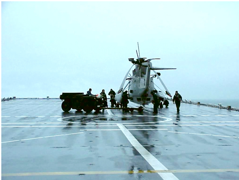
Fig. 11 Positioning the helicopter for a stern take-off following the aft/fore procedures
