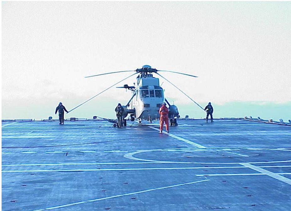
Fig. 5A Helicopter blades are unfolded automatically. To avoid blade damage, manual support is deemed essential
