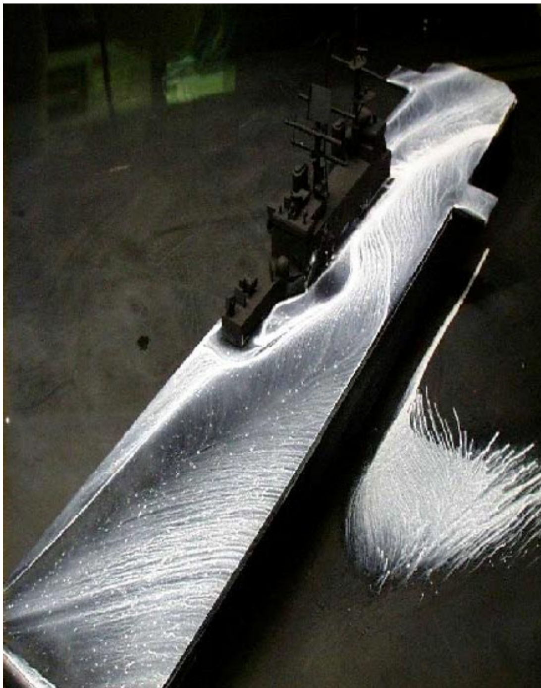
Fig. 16 Wind Tunnel Oil Flow Patterns on LHD Flight Deck
