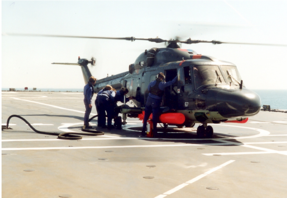
Fig. 6 Rotor Running Refuelling (Hot refuelling )
