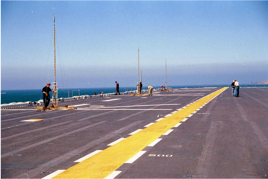
Fig. 21 JSHIP Ship Airwake Measurement System on LHA 5
