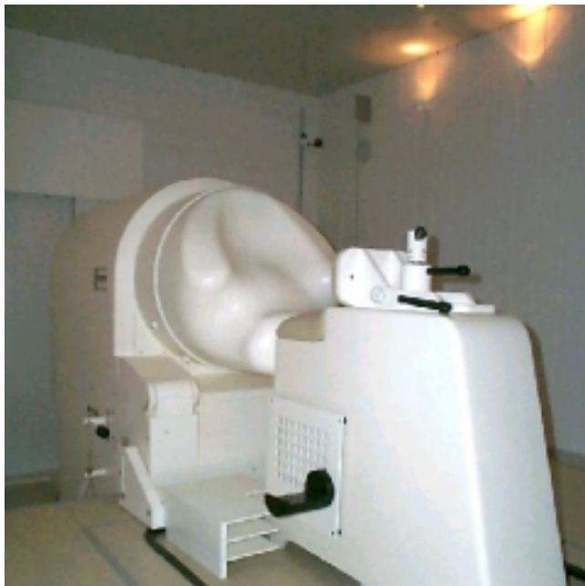
Fig. 1. The SARA system including the adjustable dewar and the patient support system.
