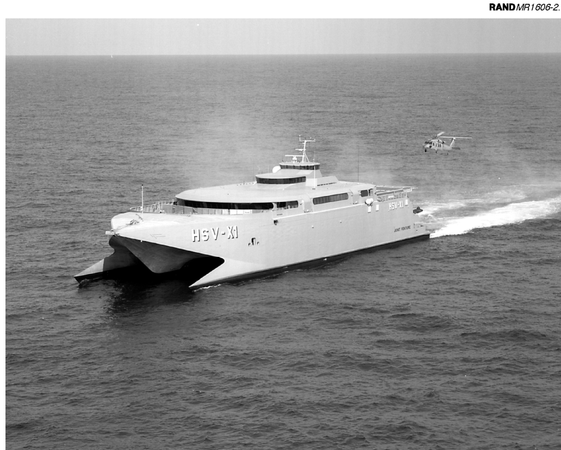
Figure 2.9—The Joint Venture , a High-Speed Catamaran Ferry Built by INCAT at Hobart, Tasmania
