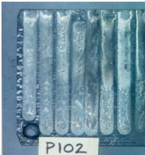
**Figure 11. Sample P102: Aluminum on Larger C-C Thermal Plane Material.**
