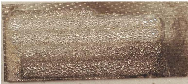
**Figure 26. Nickel Alloy Cladding Using Single-Direction Rastering.**
