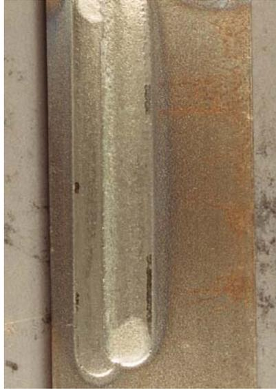
**Figure 24. Nickel Chromium Alloy Clad on Steel.**
