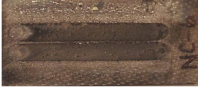
Figure 30. Alumina Powder Clad Over NiCr Alloy on C-C Substrate.
