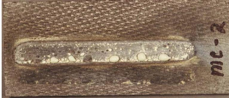
**Figure 28. Magnesium Oxide/Zirconium Oxide on C-C Substrate.**
