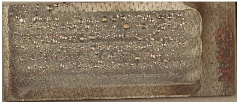
**Figure 25. Nickel Alloy Cladding Using Bi-directional Passes.**
