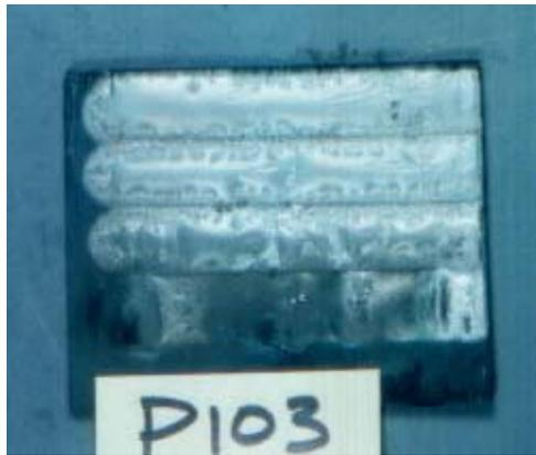
**Figure 12. Sample P103: Aluminum on Nondensified C-C.**
