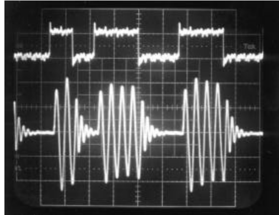
Figure 3. Suspended carrier waveform. Upper: Modulation signal. Lower: Transmitter coil current at 1A/div., 5usec/div.
