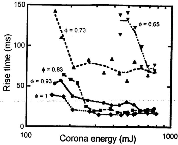
Figure 5. Rise time of corona-ignited flames as a function of discharge energy for varying values of the equivalence ratio ( $\phi$ ) of CH<sub>4</sub>-air mixtures at 1 atm with plain electrode. The maximum corona energy shown ( $\approx 800$  mJ) corresponds to the threshold beyond which arcing occurs for our geometry.
