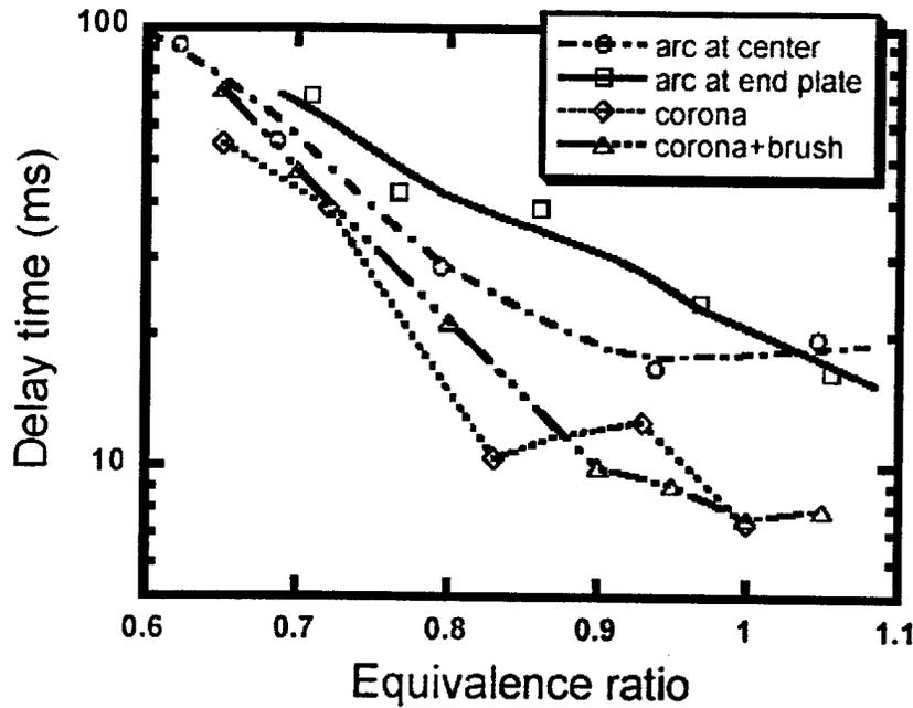
Figure 6. Characteristics of corona-ignited and arc-ignited CH<sub>4</sub>-air flames at 1 atm as a function of equivalence ratio. (a) delay time
