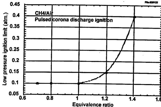
Fig.10 Low pressure limits versus equivalence ratio
