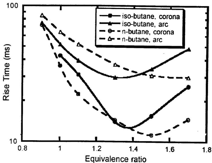
Figure 8. Rise times of corona-ignited (plain electrode) and arc-ignited (central ignition) n-C<sub>4</sub>H<sub>10</sub>-air and iso-C<sub>4</sub>H<sub>10</sub>-air flames at 1 atm as a function of equivalence ratio. Delay times (not shown) were nearly identical for all 4 cases.
