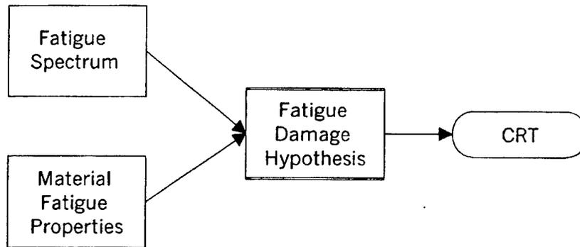
Figure 1: Simplistic representation of the safe-life methodology
