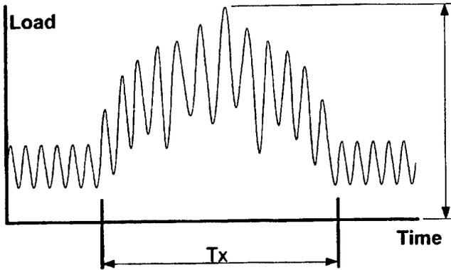
(a) Loads measured during hypothetical flight condition X, which occurs over time period  $T_x$  and which has a peak load  $L_p$  as shown.
