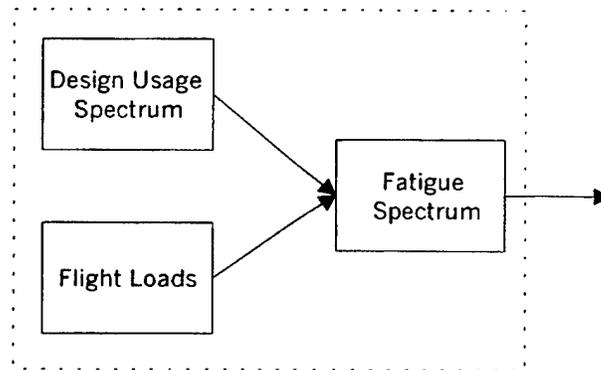
Figure 2: Inside the "Fatigue Spectrum" box of Figure. 1
