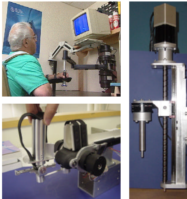
Fig.1. A Gym of Robots. The top left corner shows a recovering stroke patient receiving upper extremity robotic therapy with MIT-MANUS. The lower left corner picture shows the wrist robot and the right figure shows the spatial module (to be added to the tip of MIT-MANUS).
