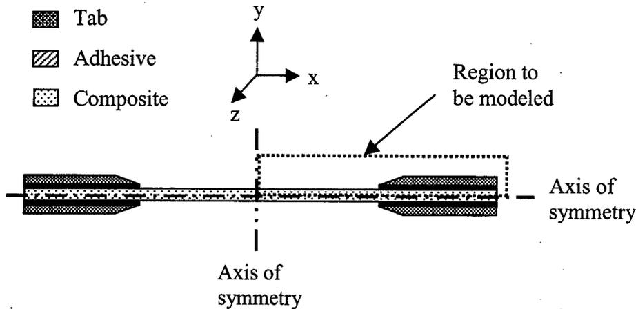
FIGURE 3. CROSS-SECTION OF SPECIMEN TO BE MODELED
