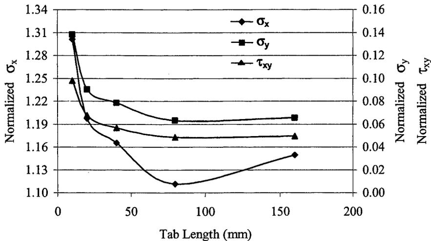
FIGURE 30. EFFECT OF TAB LENGTH ON STRESS CONCENTRATIONS IN THE COMPOSITE COMPRESSION SPECIMEN, TAPERED TAB-THIN ADHESIVE CONFIGURATION
