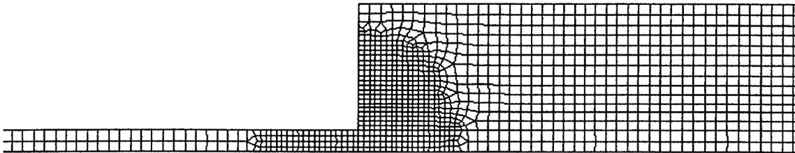
FIGURE 5b. FINITE ELEMENT MESH IN THE TAB TERMINATION REGION,
