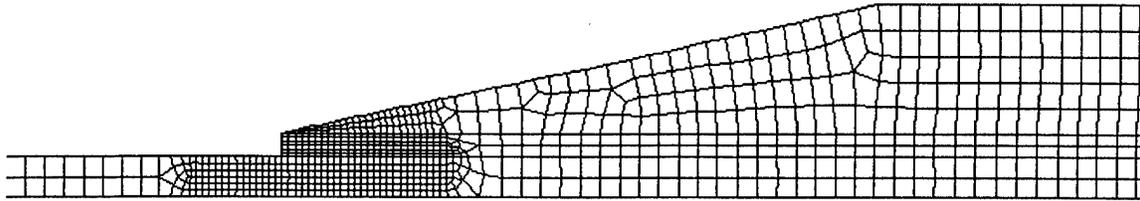
FIGURE 5a. FINITE ELEMENT MESH IN THE TAB TERMINATION REGION,
