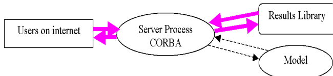
Fig. 5: The performance solution: rip out the existing MATLAB model and replace it with a five-dimensional interpolation table (results library).
