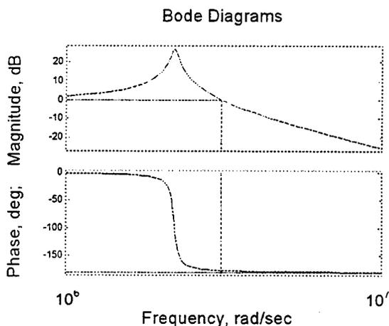
Fig. III. 2. Bode plot of the RIN model
