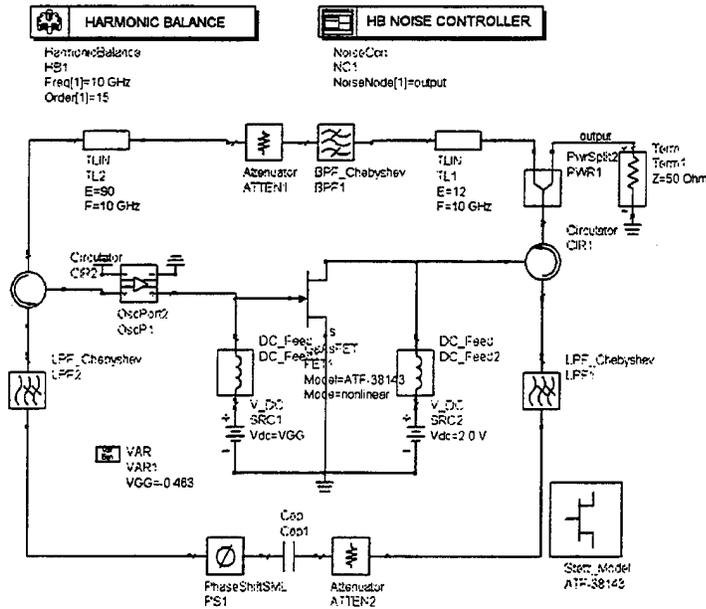
Fig. II. 4. Simulation setup for phase noise suppression
