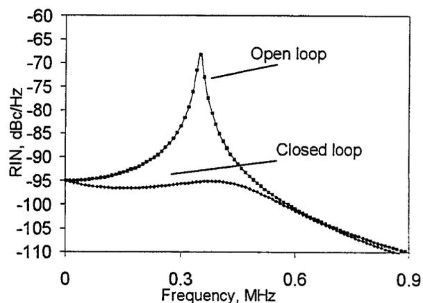
Fig. III. 3. Simulation results of RIN suppression
