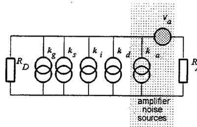
Fig. I. 6. Noise sources in the fiber-radio system
