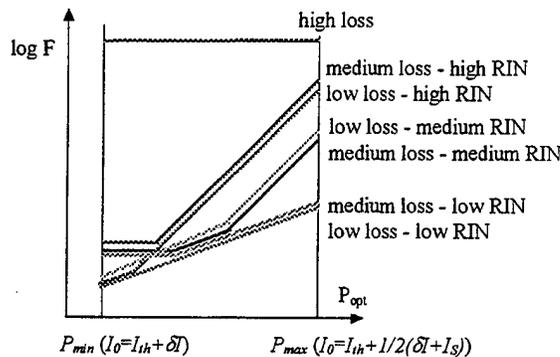
Fig. I. 7. Noise figure in special cases
