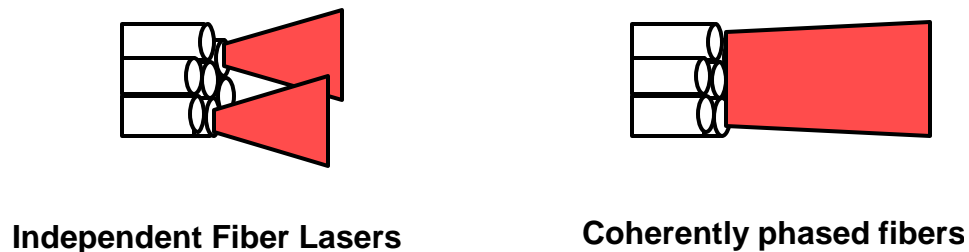
Figure 44. A Beam from an Array of Independent Fibers and a Beam from Coherently Phased Fibers.(From [Ref. 2]).
