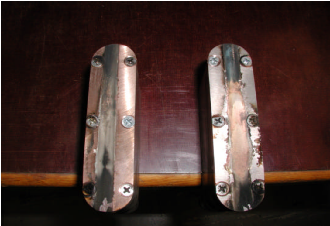
Figure 3. Rail Erosion due to 5.5 kV Discharge from Power Supply Capacitors
