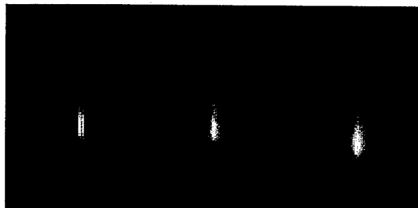
Figure 2.2 Pictures of laser sparks in quiescent air for (left) 13 \text{ mJ}/1 \pm 0.5 \text{ mm}^3 , (middle) 127 \text{ mJ}/1.3 \pm 0.7 \text{ mm}^3 , and (right) 258 \text{ mJ}/3 \pm 1 \text{ mm}^3 . Laser incidence is from bottom to top.
