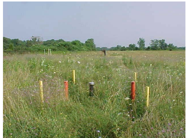
Figure 1. Monitoring wells for evaluating the reactive and hydraulic performance of a PRB at Seneca Army Depot.
