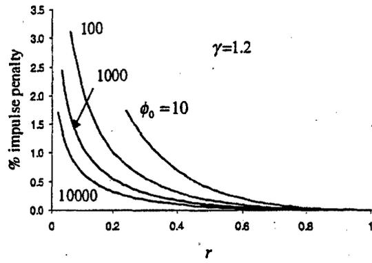
Fig. 10. Impulse penalty of an optimized fixed nozzle compared to a variable nozzle.
