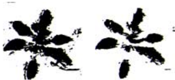
Fig. 7. Influence of threshold level in the proposed method on the area of interest: TH=30, W \times W=31 \times 31 (left), TH=60, W \times W=31 \times 31 (right)
