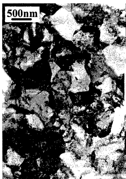
Fig. 42. Fine structure (a) and microstructure (b) of uniform SMC processed billet (150 mm in diameter and 200 mm in length) out of Ti-6Al-4V alloy.
