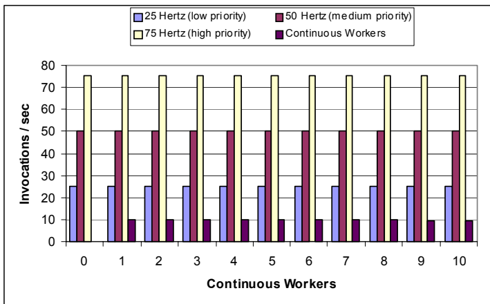
Result B: Increasing Best Effort Work in RT-CORBA With Lanes System Running Slightly Below Capacity (Work = 28)
