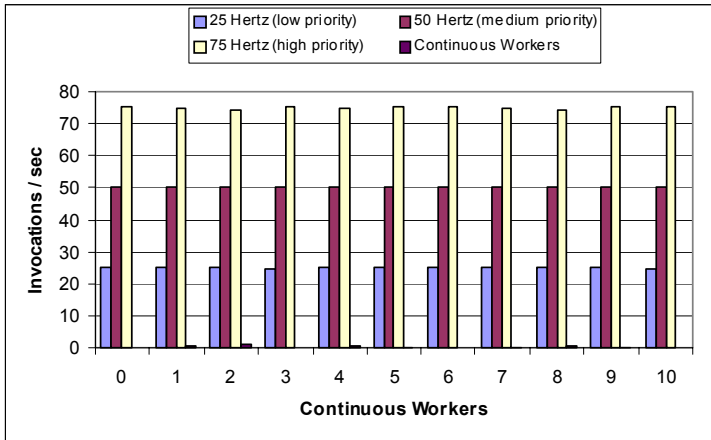
Result B: Increasing Best Effort Work in RT-CORBA With Lanes System Running Slightly Below Capacity (Work = 28)
