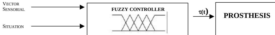
Figure 3 – Structures of fuzzy Control used for the prosthesis
