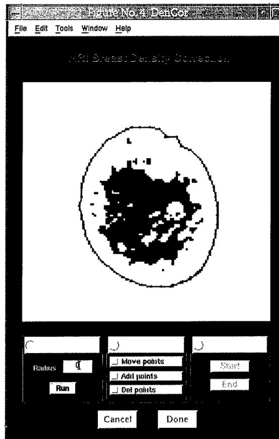
Fig. 4. The fourth screen of the GUI. After edge detection, background correction, and thresholding, the user can generate a “density mask” to define the region where the thresholded black voxels representing the fibroglandular tissue should be summed. The mask excludes the skin layer from the black voxels by applying morphological erosion to the breast boundary.
