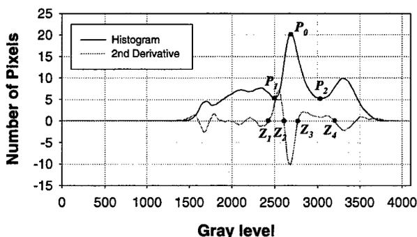
FIG. 4. The gray level histogram (solid curve) and the second derivative (dot) curve.  $P_0$  is the peak point,  $P_1$  and  $P_2$  are the valley points of the peak on the two sides of the peak point  $P_0$ . Points  $Z_1, Z_2, Z_3$  and  $Z_4$  are zero crossing points on the second derivative curve, which are used for searching the points  $P_0, P_1$  and  $P_2$ .
