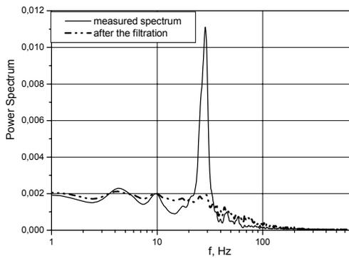
Fig. 2. Normalized power spectrum of velocity fluctuations.
