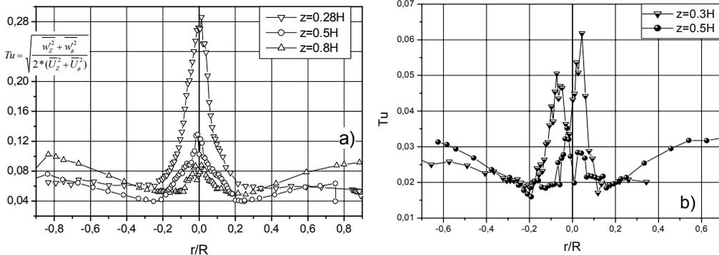
Fig. 4. The distributions of turbulence level in different cross-sections of the vortex chamber: injection of the air jet through the annular slot (a), and through the nozzle with  $d=9$  mm (b).
