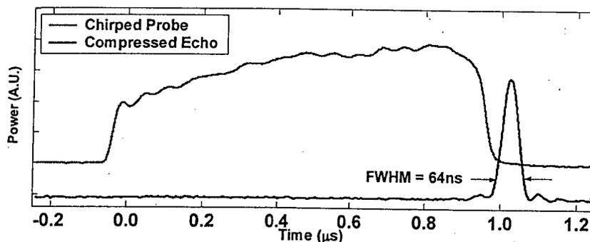
Fig. 7-4 Test of chirped pulse compression. A  $1\ \mu\text{s}$ ,  $20\ \text{MHz}$  chirp was diffracted off a chirp compressing grating producing the narrow echo. The full width half max of the echo measured at one quarter the intensity is  $64\ \text{ns}$ , close to the bandwidth limit. The probe and echo are plotted on different scales.
