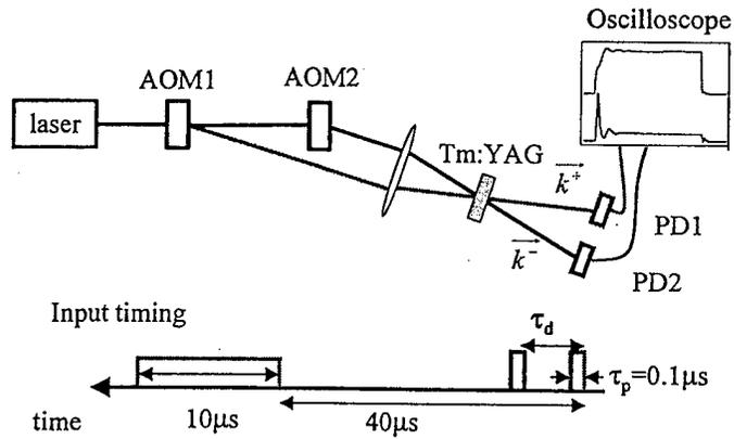
Fig. 6-3 Schematics of experimental setup and timing of the input pulses. The two programming pulses ( $0.1 \mu\text{s}$  each) are separated by a delay,  $\tau_d$ , the first incident along  $\vec{k}_+$  and the second along  $\vec{k}_-$ . The  $10\mu\text{s}$  probe is set either along  $\vec{k}_+$  to observe the echoes in the causal direction,  $\vec{k}_-$ , or along  $\vec{k}_-$  to see the echoes in the non-causal direction,  $\vec{k}_+$ .
