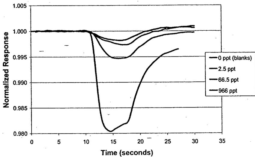
Figure 12. TNT Headspace Over Soil Standards - Time Response
