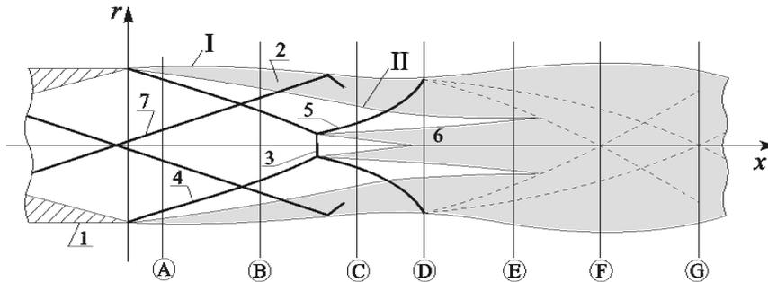
Fig. 3. Scheme of the supersonic over-expanded jet.
