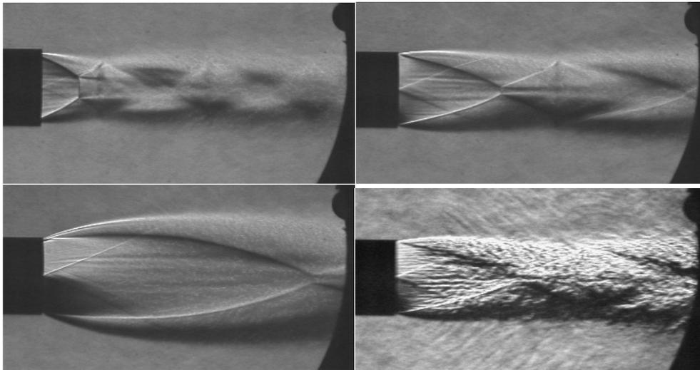
Fig. 2. Schlieren pictures of the supersonic non-isobaric jet taken with a long exposure time (1/30 s) for the pressure ratios  $n=0.303$  (left top),  $n=0.748$  (right top), and  $n=2.314$  (left bottom) and with the short exposure time for  $n = 0.785$  (right bottom).
