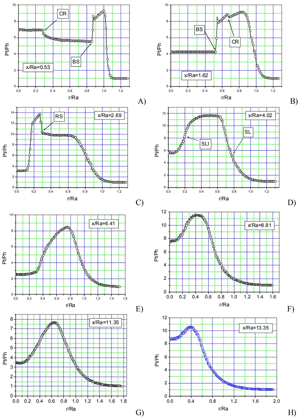
Fig. 5. Radial distribution of the Pitot pressure in the supersonic over-expanded jet measured in various jet cross-sections,  $M_a = 3.005$ ,  $n = P_a/P_t = 0.6$ .
