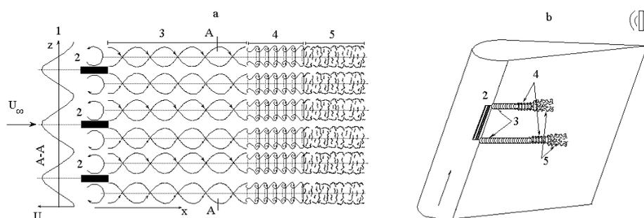
Fig. 1. Schemes of the transition in the flat plate (a) [9] and swept wing (b) [12] boundary layers modulated by streamwise structures. 1 – spanwise velocity distribution; 2 – roughness elements; 3 – streamwise structures; 4 – secondary disturbances; 5 – turbulence. Secondary disturbances were excited by vibrating ribbon (a), acoustic and blowig-suction (b).
