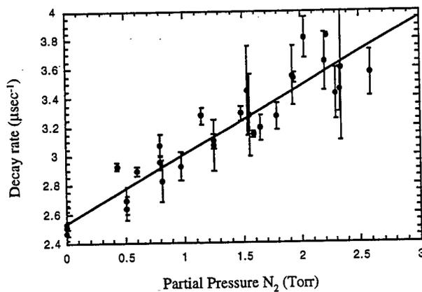
Figure 4 Pressure dependence of decay rate for N<sub>2</sub> collider (plus 1.2 T CO, plus 4 T helium buffer gas). See text for explanation of error bars.
