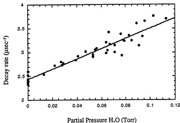
Figure 5 Pressure dependence of decay rate for H<sub>2</sub>O collider (plus 1.2 T CO, plus 4 T helium buffer gas).
