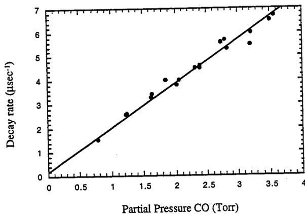
Figure 3 Pressure dependence of decay rate for CO collider (plus 4 T helium buffer gas).
