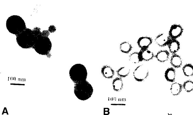
Figure 3. Transmission electron micrographs of A.) gold-silicate core-shell particles containing 15 molecules of Cascade Blue per particle or 243 molecules of Sulforhodamine-G per particles. B.) After removal of the 85 nm diameter colloidal gold core
