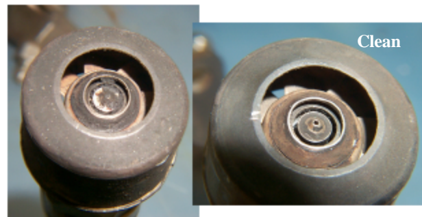
Figure 8 – Clean Nozzle and One with Severe Clogging
