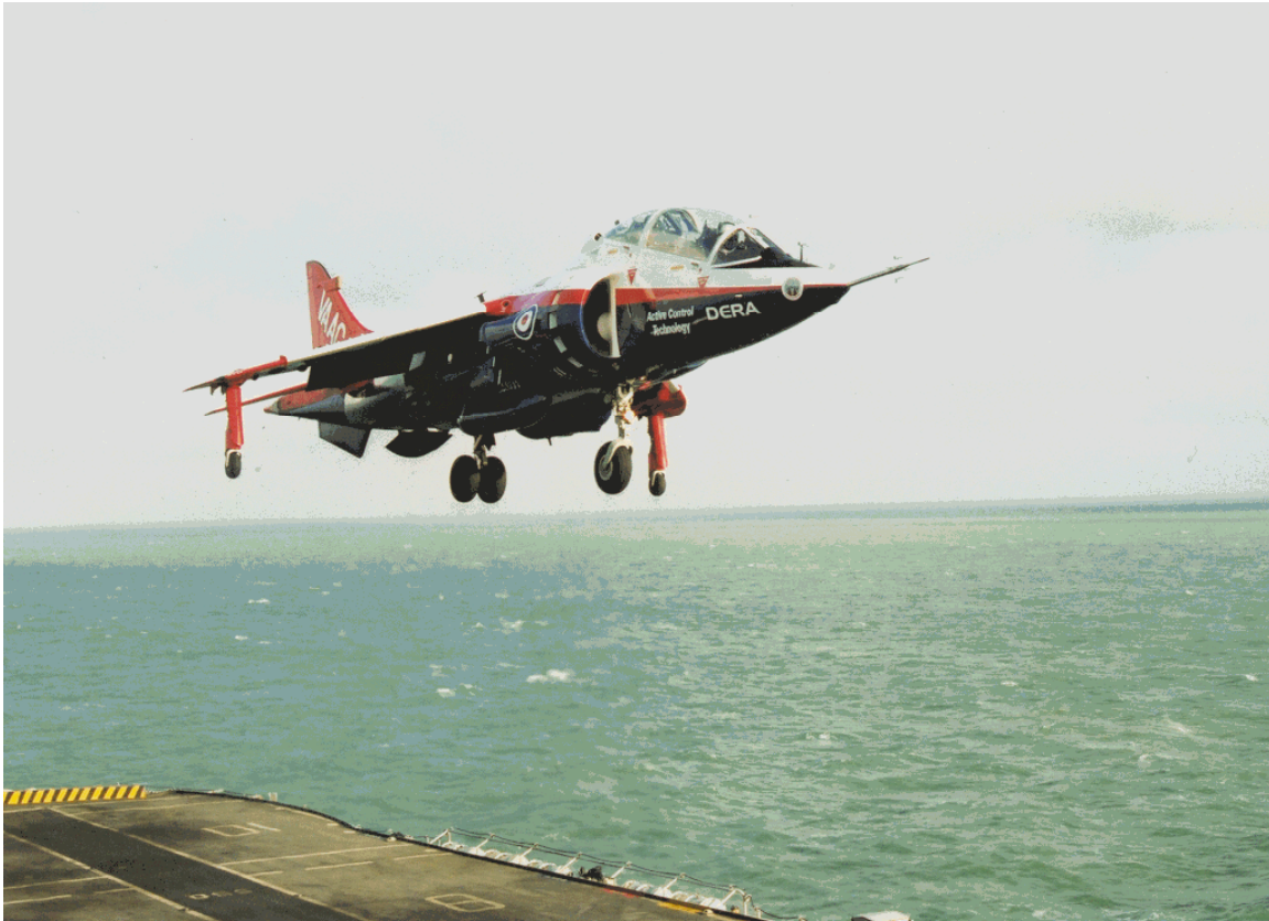
Figure 4.9 - Harrier STOVL aircraft maintaining attitude control in hovering flight using control thrusters
