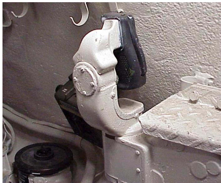
Fig III.14 - The M47 commander's turret elevation control moves in pitch, but rotates in yaw to control traverse.
