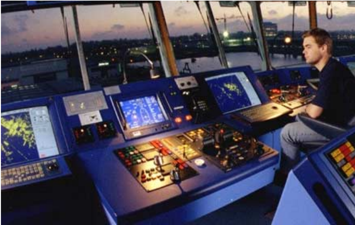
Fig. 5.8 - Typical Integrated Bridge System arrangement (Kongsberg Maritime Ship Systems (KMSS) Bridgeline series).
