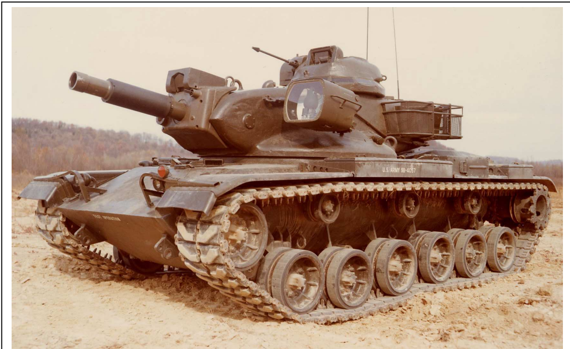
Fig III.17 - A US M60A2 tank. The large commander's cupola was independently stabilized in elevation and traverse. Upon acquiring a target, the commander could engage it with the .50-caliber machinegun, or could take control of the turret and "auto-align" the main weapon to the target currently in the cupola crosshairs. The commander's cupola controls could also be used to fire the primary armament in the event the tank was operated with a three-man crew, without the gunner. In practice, the workload on the combined commander/gunner was significantly increased, and this practice was not seen as a favorable indicator of desirability of a reduced crew.
