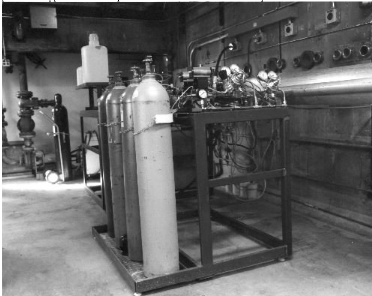
Figure 17. Photograph of oxygen supply and pressurization subsystem
