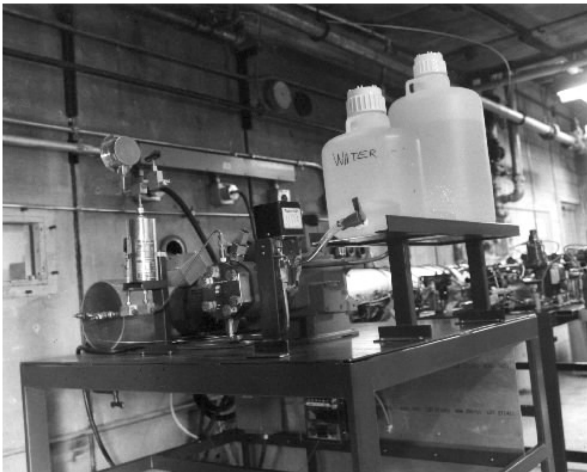
Figure 16. Photograph of wastewater feed and pressurization subsystem
