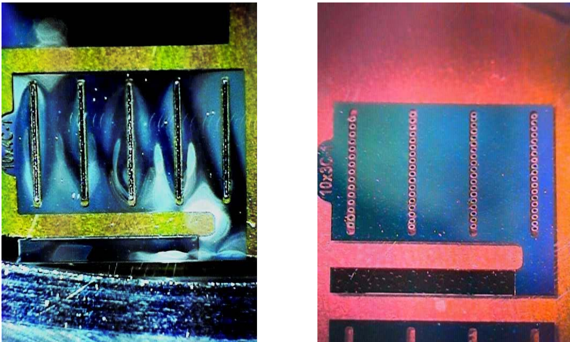
Figure 45. Long slits cut in a polymer sheet, showing the distortion near the slit edges. Rows of laser-cut holes eliminate the distortion. These devices were assembled using the technique shown in Figure 47A, appropriate for single layer actuators.
